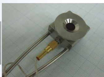
QCM sensor for detection of VOC molecules and active oxygen
